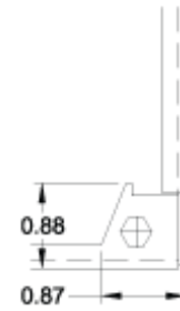
Hinge Detail Retractable pin allows door to be mount on left side or right side.
