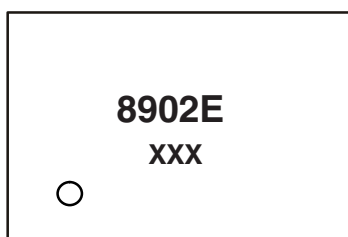
Mark on Backside of Die
