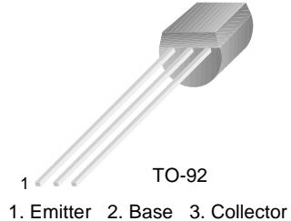
**NPN Epitaxial Silicon Transistor****Absolute Maximum Ratings**  $T_a=25^\circ\text{C}$  unless otherwise noted
