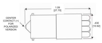
Measurements are typical Dimensions are inches [mm]
