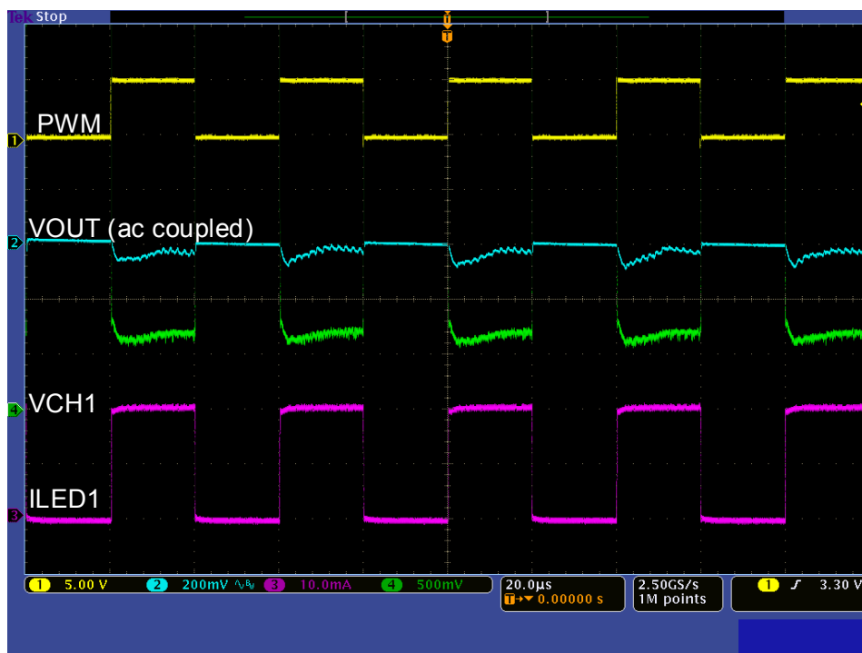
Figure 8. Typical Operating Waveforms (FPWM = 25 kHz, 50% duty)
