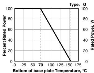
Best results can be reached by using a thermal transfer compound with a heat conductivity of better than 1W/mK
