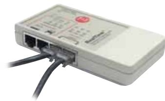
AX-110BT Realtime 10/100 Base-TX Ethernet Network Test Unit
