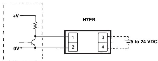
Note: When using H7ER-SBV, connect an external power supply as shown by the dotted line. Other than that, do not connect or use terminals ③ or ④ for any reason.
