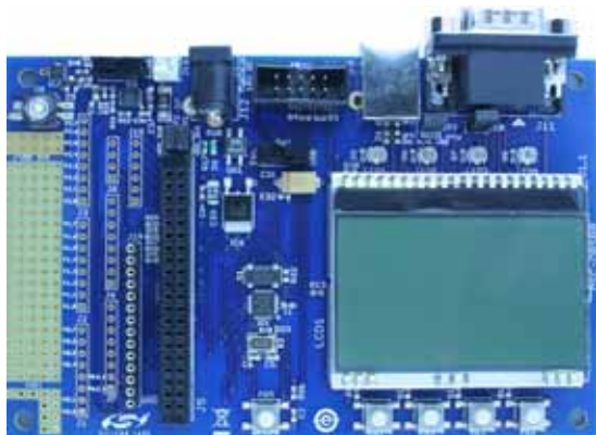
Figure 1. MSC-DBSB8 Software Development Board (SDB)
