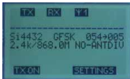
Figure 21. Non-Antenna Diversity Testcard
