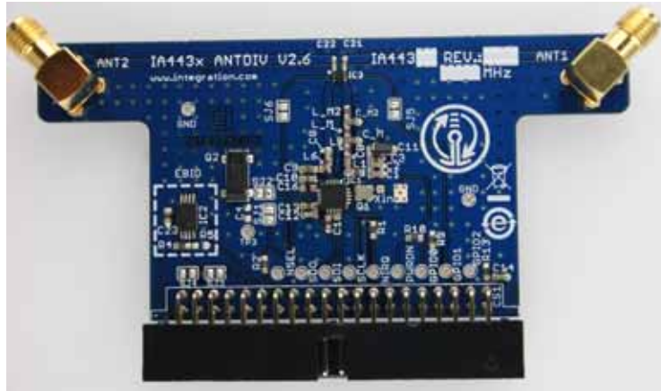
Figure 15. Antenna Diversity Testcard (May be Ordered Separately)
