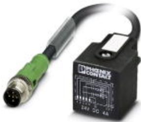
Sensor/Actuator cable, 5-position, PUR halogen-free, Black RAL 9005, Plug straight M12 SPEEDCON, A-coded, on Valve connector AD (pressure switch), with 2 LEDs, Cable length: 0.6 m
