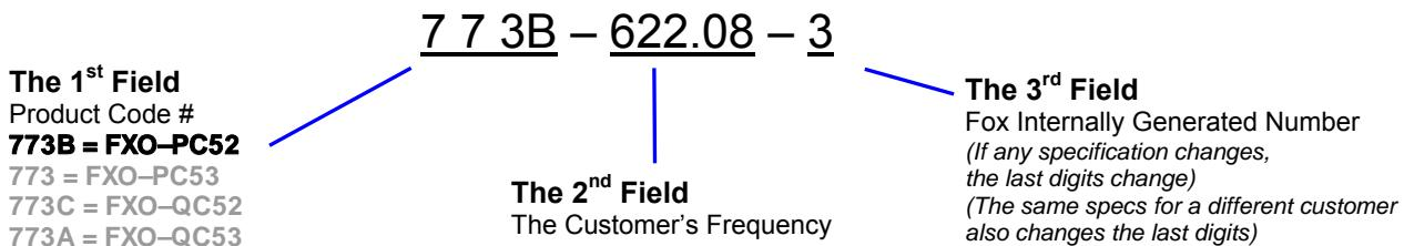
This example, **FXO-PC526R-622.08** = LVPECL Output, Ceramic, 5 x 3.2mm Package, 2.5V, ±25 PPM Stability, -40 to +85°C Temperature Range, at 622.08 MHz
