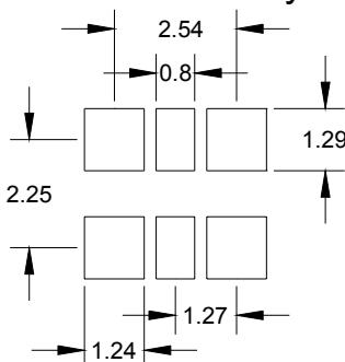
Note: XPRESSO LVPECL XOs are designed to fit on Industry standard, 6 pad, layouts.
