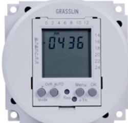
The FM1D20-120U One-Circuit Electronic Time Switches are compact electronic 24-Hour/7-Day modules with heavy-duty relay contacts for switching low or line voltage loads. The timers are applicable for time-of-day control of pumps, fans, heaters, HVAC control circuits, lighting, machinery and many other types of commercial, industrial and agricultural equipment.
