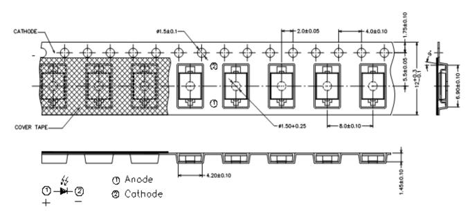
**Note:** The tolerances unless mentioned are ±0.1 mm, unit: mm.
