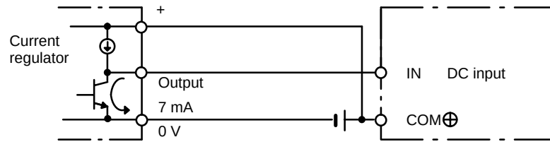
NPN open-collector output
