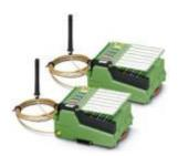
Wireless MUX set, consisting of two modules with 16 digital inputs and outputs and two analog inputs and outputs each, as well as two OMNI antennas, transmission power 8 dBm, antenna gain 2 dBi
