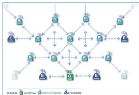
IP-Link 3000& 3200 dongles support Star, Cluster-Tree and Mesh Topologies
