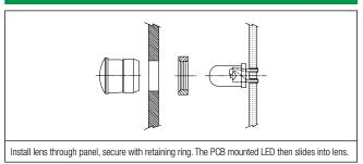
CLIPLITE® lenses, installed in a display panel, are used with PCB mounted LEDS. Lenses remain attached to the display or panel door while the LEDs are fixed to the PCB. The lenses are ideal when used together with the CONXRITE  $^{\scriptsize \odot}$  connector assembly.
