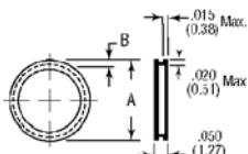
Suggested for sealing connectors to protect from vibration and moisture. Grey elastomer.
