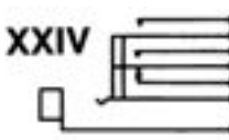
Single open circuit. Isolated switching—separate transfer and "make" circuits. (J1-1A-1C).
