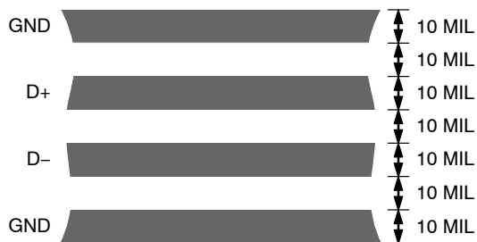
Figure 18. Typical Arrangement of Signal Tracks
