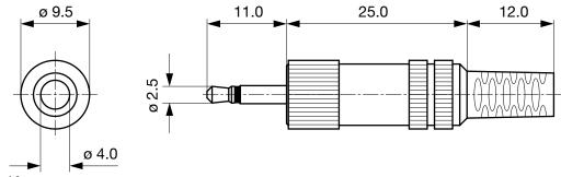
Cable diameter max. 4.0 mm
