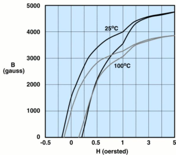
Measured on an 18/10/6mm toroid at 10kHz.
