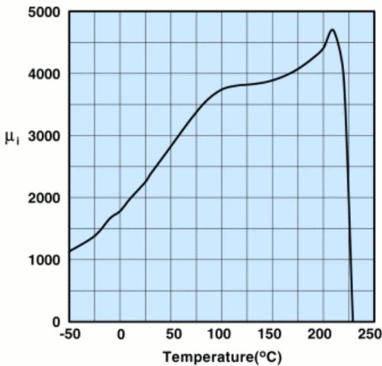
Measured on an 18/10/6mm toroid at 100kHz.
