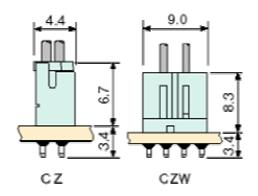
With the CZ receptacles and headers, and v holder and its mating headers, highly dense design is possible.
