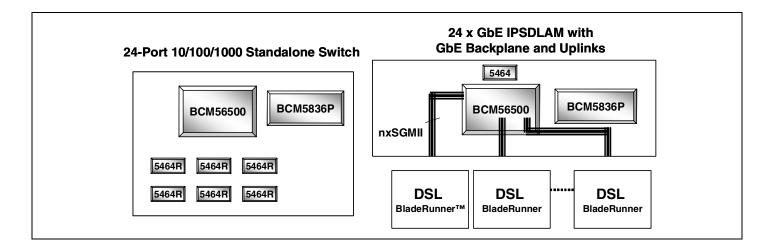
The BCM56500 is the fifth generation of the highly-integrated and cost-effective StrataSwitch and StrataXGS product line in a single-chip solution with 24-GbE ports. The BCM56500 incorporates 24-GbE ports that can operate 10/100/1000 Mbps.
