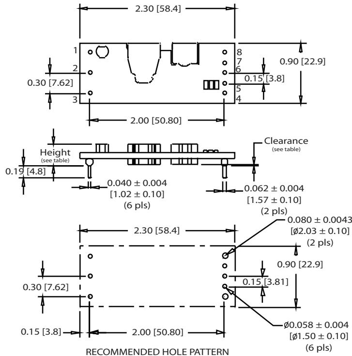
Surface-mount Mechanical Drawing (for 2.5, 3.3, 6 and 12 V)
