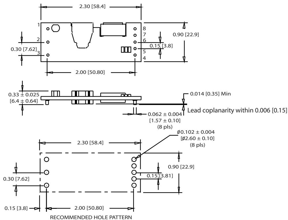
Through-hole Mechanical Drawing (for 2.5, 3.3, 6 and 12 V)
