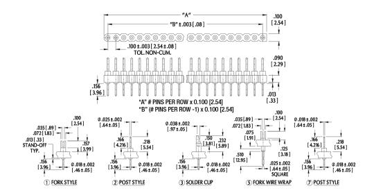
ALL DIMENSIONS: INCHES [MILLIMETERS] ALL TOLERANCES: ±0.005 [0.13] UNLESS OTHERWISE SPECIFIED FOR COINED CONTACTS, SEE DATA SHEET 12034 **CONSULT FACTORY FOR OTHER SIZES AND CONFIGURATIONS**
