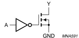
Fig.4 Logic diagram.
