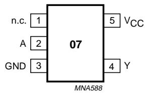
Fig.1 Pin configuration.
