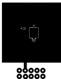
a. 57 °C/W when mounted on a 1 in 2 pad of 2 oz copper
