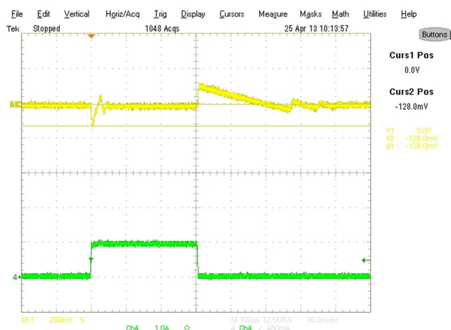
Fig. 11: Load Step Response 10mA to 800mA V_{IN}=3.3V , V_{OUT}=1.8V , C_{IN}=10\mu F , C_{OUT}=22\mu F Ceramic ch1= V_{OUT} , ch4= I_{LOAD} , time=100us/div
