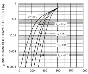
V<sub>F</sub>, INSTANTANEOUS FORWARD VOLTAGE (mV) Fig. 2 Typical Forward Characteristics
