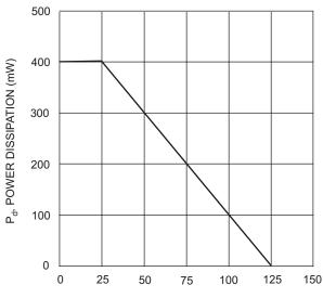
T<sub>A</sub>, AMBIENT TEMPERATURE (°C) Fig.1 Power Derating Curve
