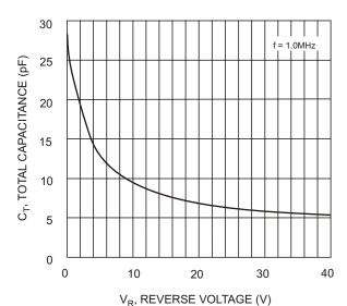
Fig. 4 Typ. Total Capacitance vs. Reverse Voltage
