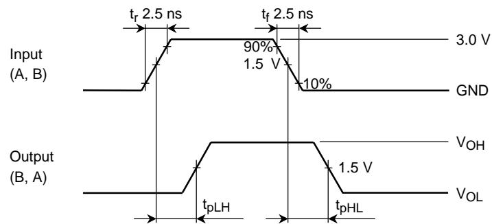
Figure 2  $t_{pLH}, t_{pHL}$
