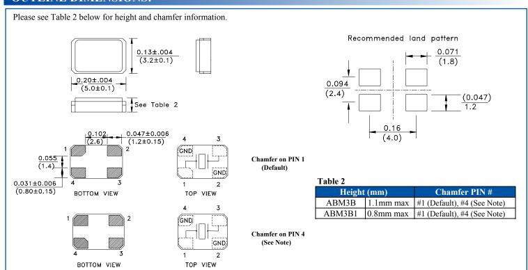
Note: Due to the availability of raw materials, this part may be manufactured with the chamfer on pin 4. Be advised that this does not affect the electrical characteristics of the crystal in any way.
