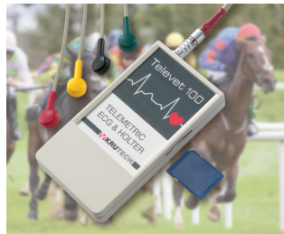
Telemetric ECG system for veterinary medicine
