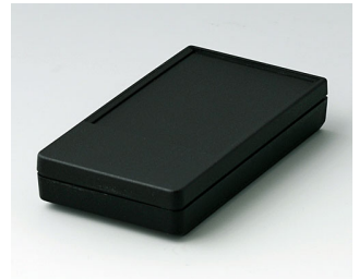
A9070119 DATEC-POCKET-BOX S ABS (UL 94 HB) black RAL 9005 3.35"x1.81"x0.63" IP 54
