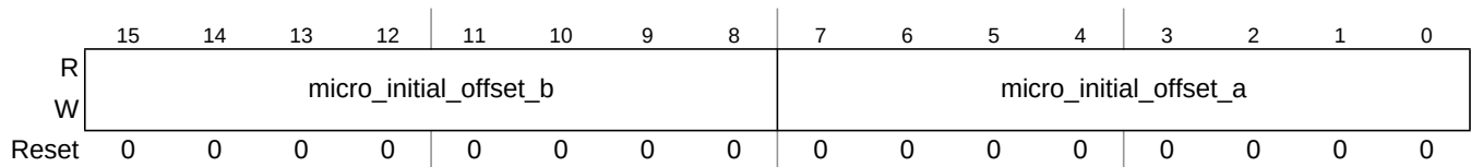
Figure 13-85. Protocol Configuration Register 20 (PCR20)
