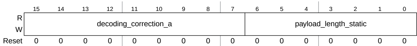
Figure 13-84. Protocol Configuration Register 19 (PCR19)
