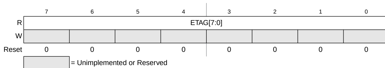
Figure 4-19. EEE Tag Counter Low Register (ETAGLO)
