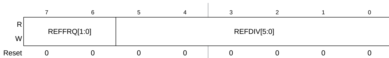
Figure 12-4. CGMIPLL Reference Divider Register (CGMREFDV)
