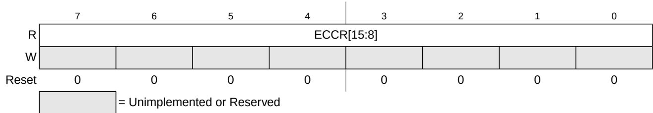
Figure 10-20. Flash ECC Error Results High Register (FECCRHI)
