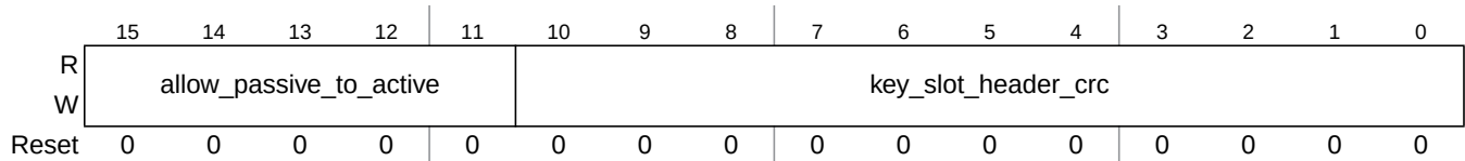
Figure 13-77. Protocol Configuration Register 12 (PCR12)
