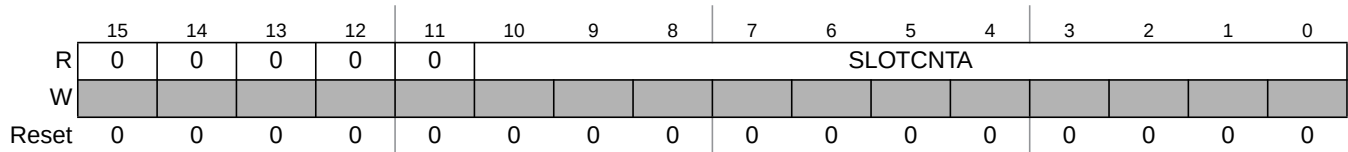
Figure 13-26. Slot Counter Channel A Register (SLTCTAR)
