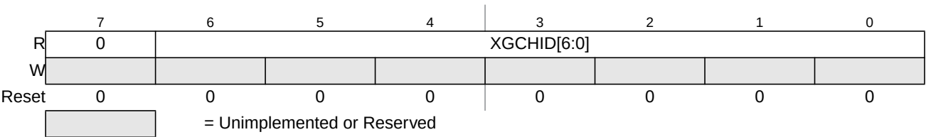
Figure 14-4. XGATE Channel ID Register (XGCHID)
