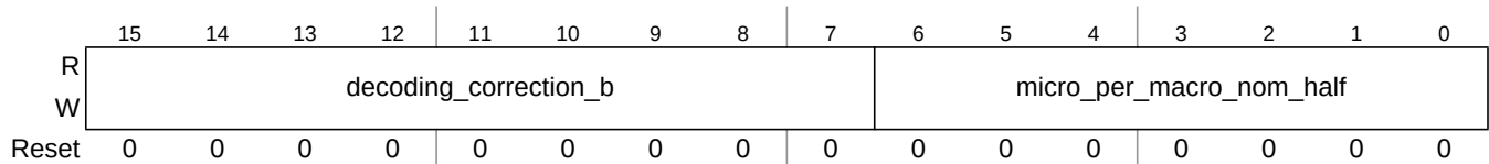
Figure 13-72. Protocol Configuration Register 7 (PCR7)
