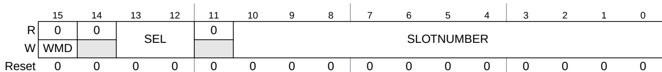
Figure 13-45. Slot Status Selection Register (SSSR)
