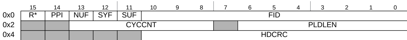
Figure 13-105. Frame Header Structure
