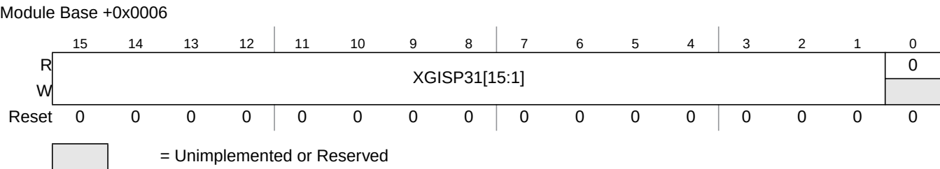
Figure 14-8. XGATE Initial Stack Pointer for Interrupt Priorities 3 to 1 (XGISP31)
