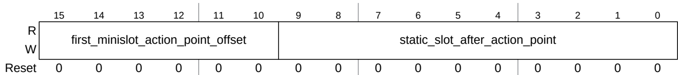
Figure 13-78. Protocol Configuration Register 13 (PCR13)
