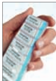
Step 2 Bend liner at side slit
