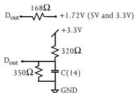
Figure C: Output load
