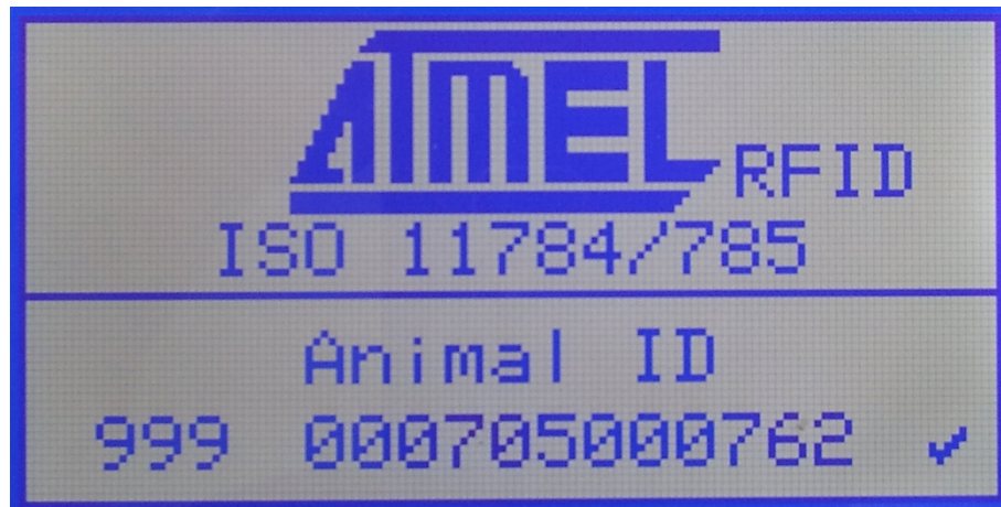
Figure 1-6. LCD Display with Animal ID Read Selection in Stand-alone Mode
