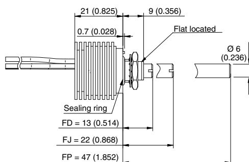
Available only with bushing M10 x 0.75 and shafts Ø 6 mm
