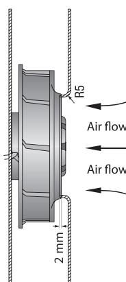
The air flow and sound level of the centrifugal fans without external housing depend on their individual installation conditions. The stated air flow and noise levels have been measured under the following conditions:
