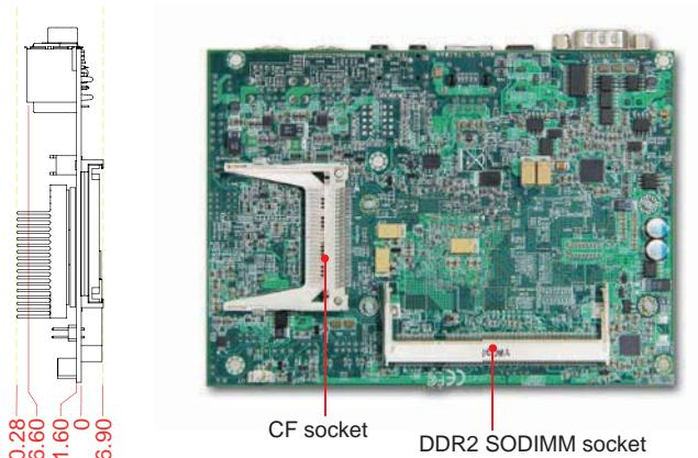
PEB-2738I takes advantage of the latest Intel® Atom™ technologies. It supports DDR2 SDRAM, one gigabit ethernet and one expansion Multi function connector. Based on leading Intel® Atom™ solution, PEB-2738I performs low power dissipation, high performance and fanless requirement. Therefore, it's applied to Panel PC, Kiosk, Medical, and industrial automation.
