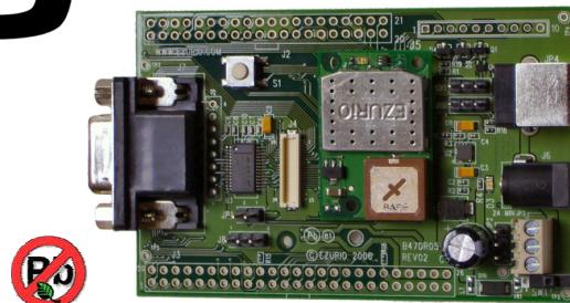
The EZURiO Development Kit is designed to support the rapid development of hardware, applications and software for the EZURiO range of BISM II Bluetooth Intelligent Serial Modules and WISM Wireless LAN modules. The EZURiO development kit is available in five options to cover the widest range of wireless technologies, including hardware support for development of applications for the Siemens MC55 GSM GPRS modules.
