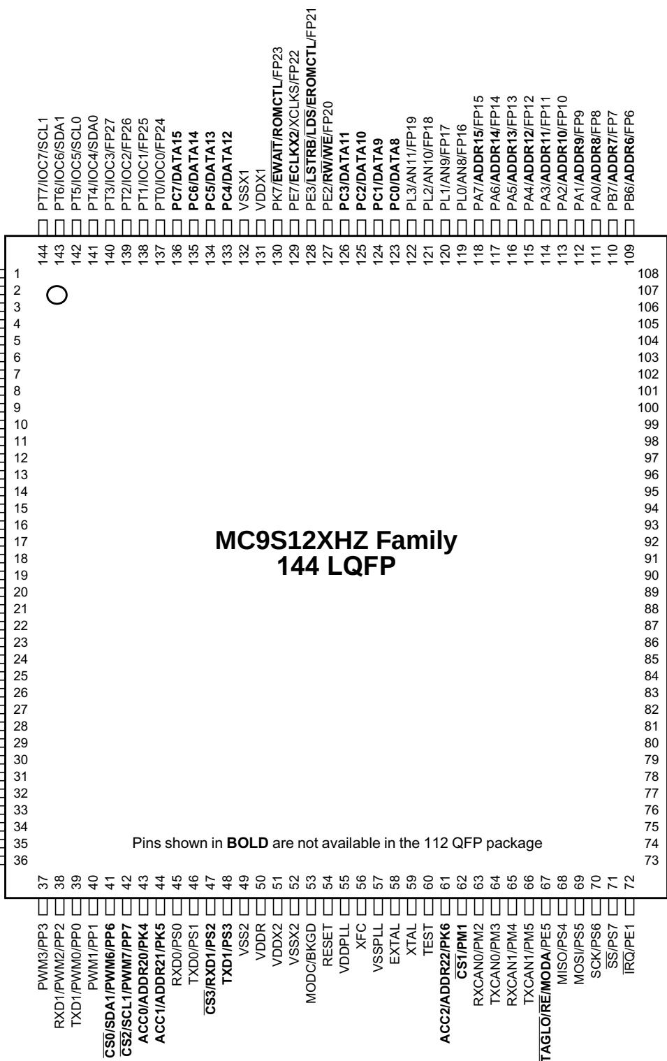
Figure 1-4. MC9S12XHZ Family 144 LQFP Pin Assignment
