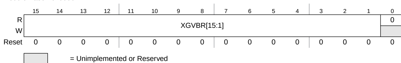
Figure 5-5. XGATE Vector Base Address Register (XGVBR)
