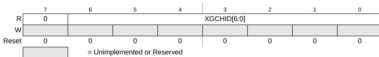
Figure 5-4. XGATE Channel ID Register (XGCHID)
