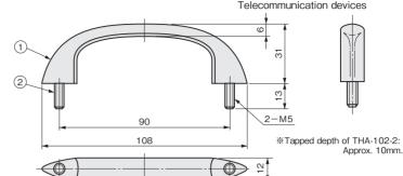
■Parts List The figure shows the pull with feet
