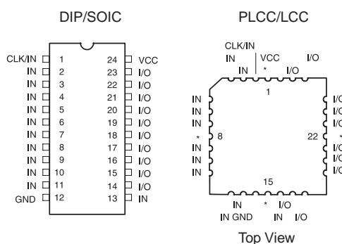
Each of the ATV750B's 22 logic pins can be used as an input. Ten of these can be used as inputs, outputs or bi-directional I/O pins. Each flip-flop is individually configurable as either D- or T-type. Each flip-flop output is fed back into the array independently. This allows burying of all the sum terms and flip-flops.
