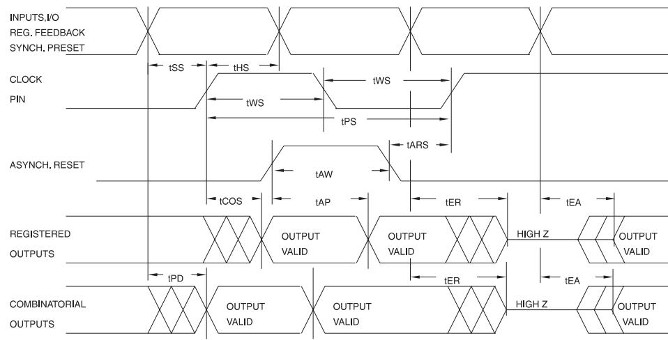
Notes: 1. Timing measurement reference is 1.5V. Input AC driving levels are 0.0V and 3.0V, unless otherwise specified.
