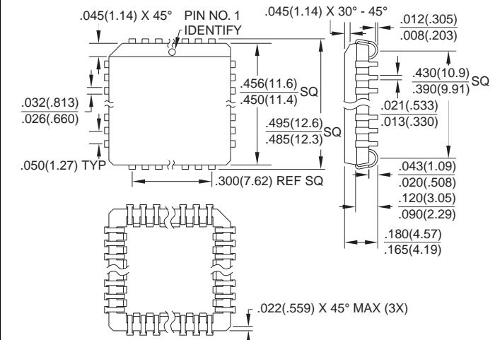
**28LW**, 28-Pad, Windowed, Ceramic Leadless Chip Carrier (LCC)
