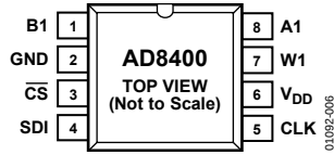
Figure 6. AD8400 Pin Configuration
