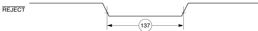
Figure 63. CAM Interface \overline{\text{REJECT}} Timing Diagram
