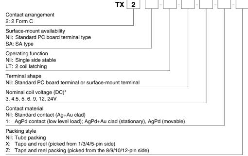
Note: In case of 5 V transistor drive circuit, it is recommended to use 4.5 V type relay.
