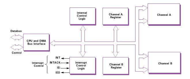
The ESCC has many improvements that significantly reduce CPU overhead. The addition of a 4-byte transmit FIFO and an 8-byte receive FIFO significantly reduces the overhead required to provide data to the transmitters, and to get data from the receivers.
