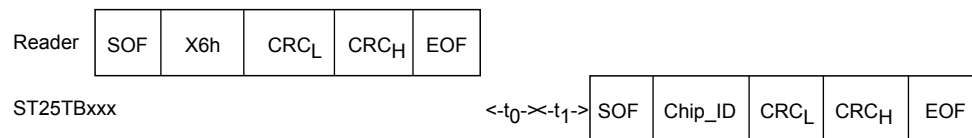
Figure 47. Slot_marker frame exchange between reader and ST25TB512-AT
