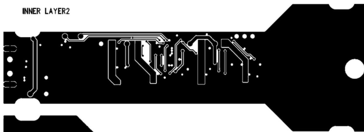
Figure 14. Front Side Inner Layer 2
